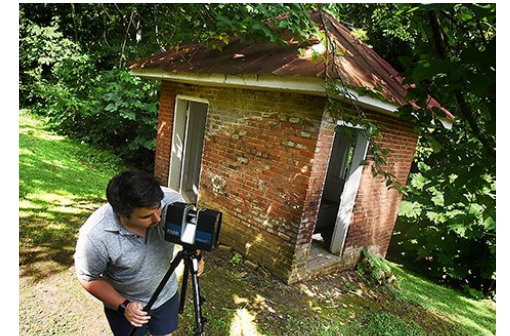
Brent Fortenberry of Texas A&M uses a combination of modern technology (drone photography and 3-D laser scanner) and centuries-old technology (pencil, paper, and measuring tape) to record the privy at Longwood. (Photo credit: Ben Hillyer, Natchez Democrat)
